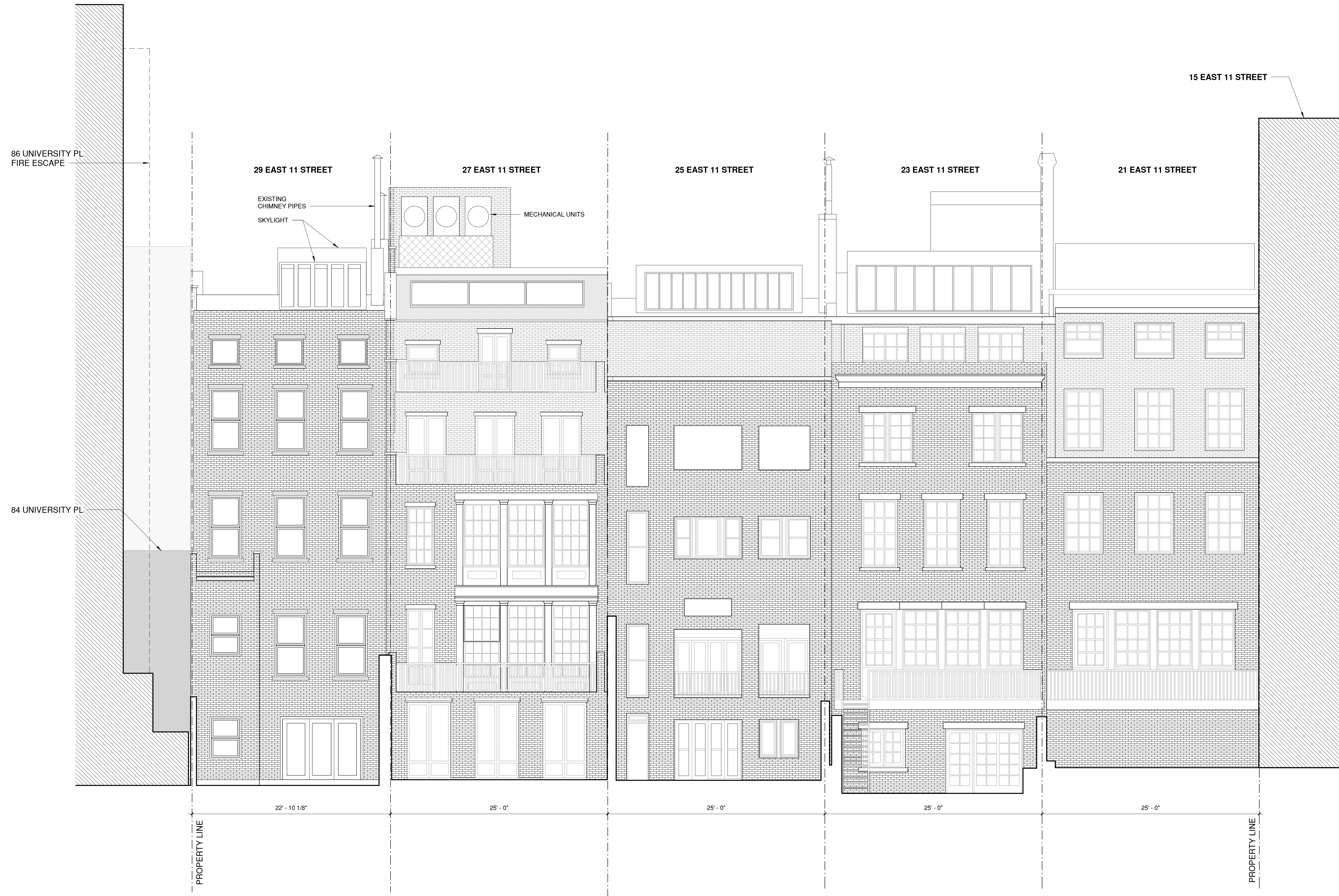
1 Row Houses Rear Elevation - Existing 3/16" = 1'-0"
